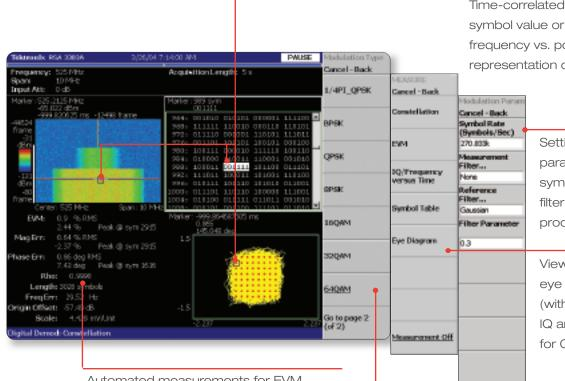
Time-correlated views relate EVM, symbol value or constellation with frequency vs. power or spectrogram representation of a digital signal
